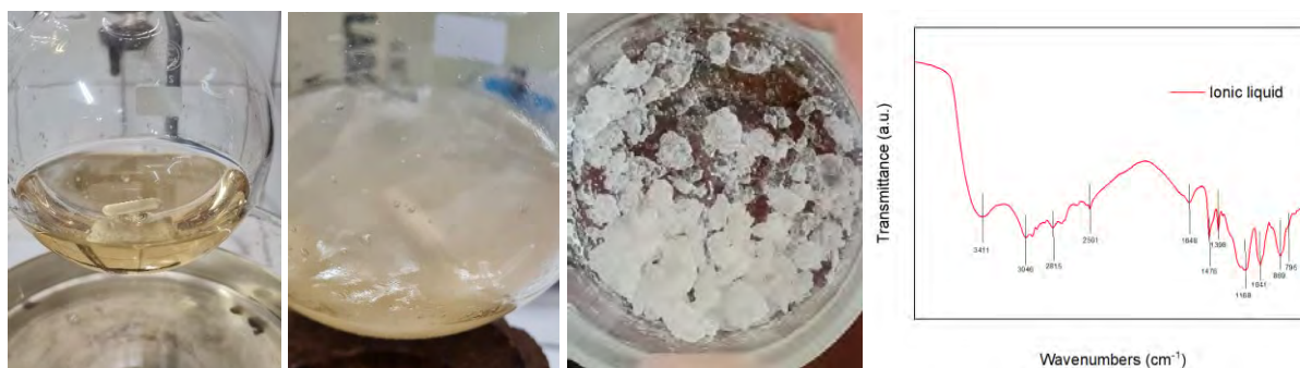
Figure 4: IL during the synthesis, cooling and precipitation phase and its FTIR spectrum
