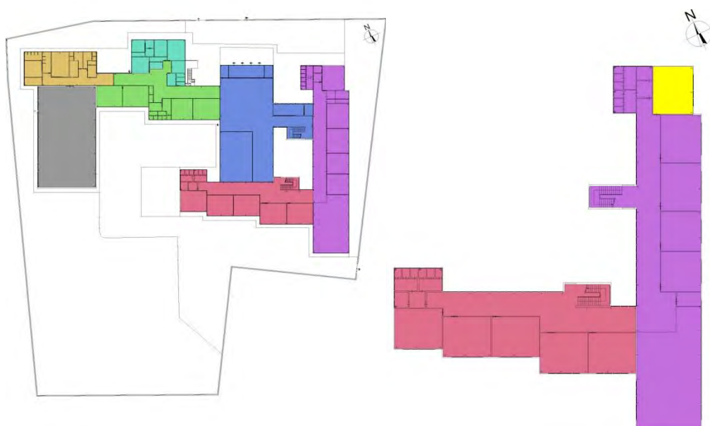
Figure 2. On the left, thermal zones at ground floor: gym (gray); changing rooms (yellow); classrooms (green); offices (light blue); hall (blue); classrooms (purple); classrooms (red). On the right, thermal zones at first floor: classrooms (purple; at the top the studied classroom highlighted in yellow); classrooms (red)
