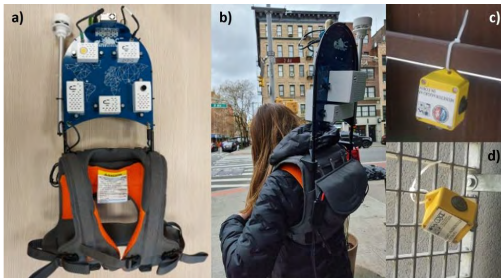
Figure 1. Monitoring devices: a and b) wearable system; c) thermohygrometer at the urban park; d) thermohygrometer at the commercial hub.
